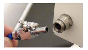
All operatories are equipped to operate ultrasonic devices. The air pressure to each operatory chair, and all the handpieces, are factory set at approximately 35 to 50 psi. Please ensure that your handpiece will operate effectively within these parameters.
