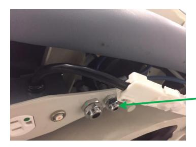
Water connection for ultrasonic scaler under right side of chair. Power outlet also in this area. Note this is the smaller connector nearest the grey knob.
